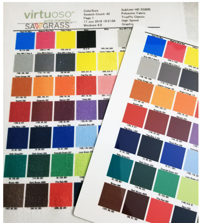
The palette on the left is pressed onto a polyester sports towel, while the one on the right is pressed onto a white ChromaLuxe photo panel.
